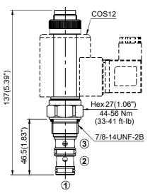
● Allowed Back Pressure at port 3 (T): 5 bar (73 psi)max. 允許背壓在孔□3 (T): 最大5bar(73psi)
